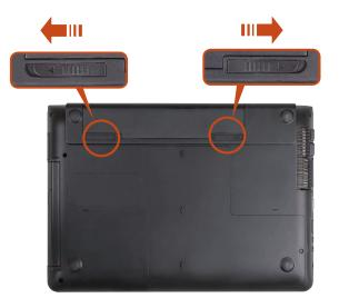
3 To install the battery again, slide the battery into the system. The battery latches move inwards and fix the battery automatically. You can connect a Kensington lock to the Security Lock port to prevent your computer from being stolen when you have to use the computer in a public place.
