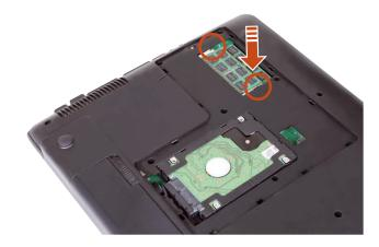
**Close the memory compartment cover and fasten the screw.**
