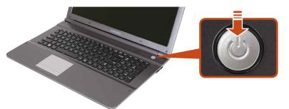
**Power button LED** is lit while the computer is turned on.
