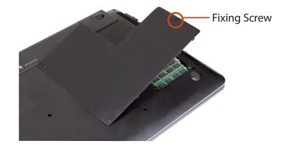
Insert a new memory module into the memory slot at an angle of approximately 30 degrees aligning it to the angle of the memory slot.
