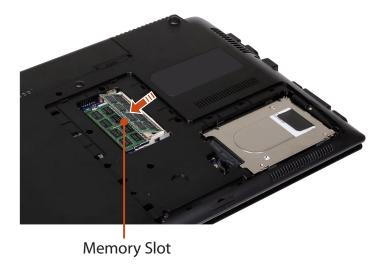
Push the memory module down so that it is completely fixed. If the memory does not fit easily, push the memory module down while pulling the memory module latches outward.
