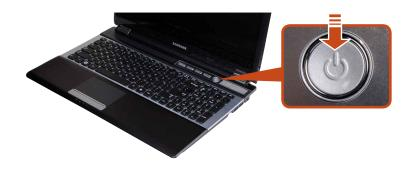
**Power button LED** is lit while the computer is turned on.
