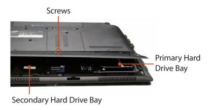
1 Insert the secondary hard drive into the case so that all the holes are lined up and then 2 fasten the hard drive screws to secure the hard drive to the case.
