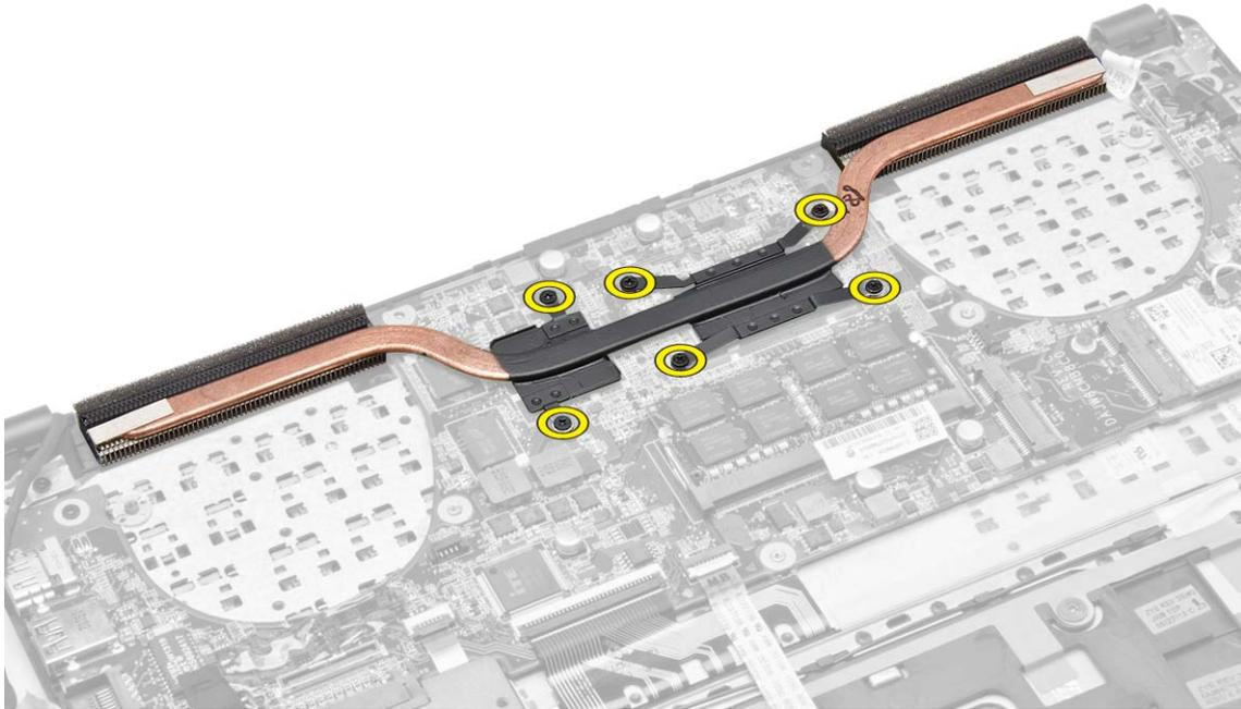
4. Lift up the heatsink and remove from the computer.
