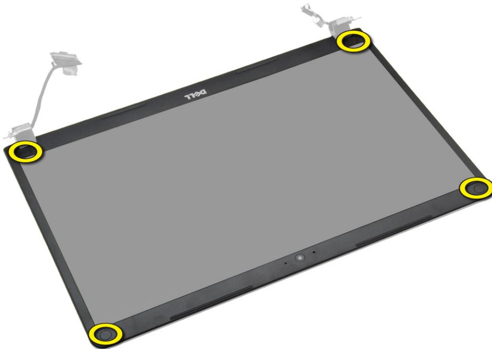
5. Remove the screws that secure the display bezel.
