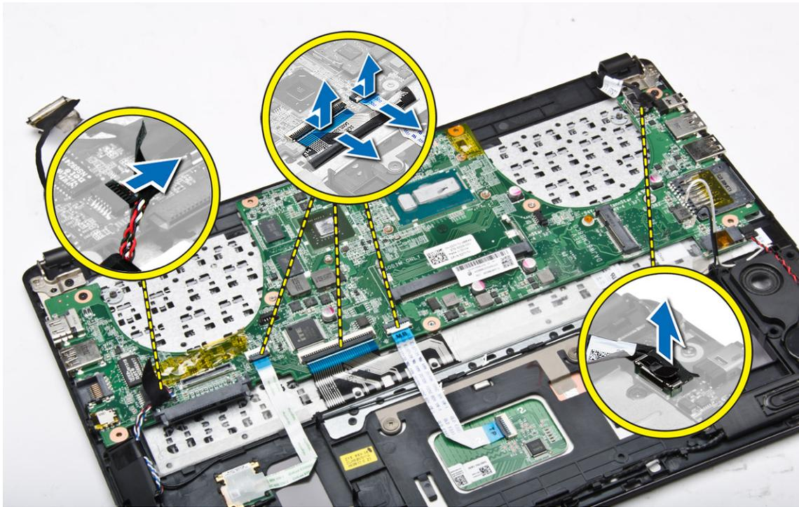
4. Remove the screws that secure the system board to the chassis.
