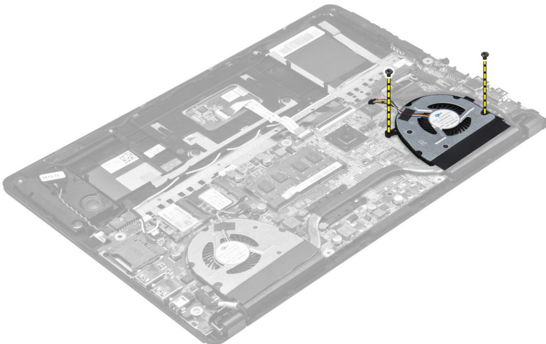
7. Lift and remove the right system fan from the computer.
