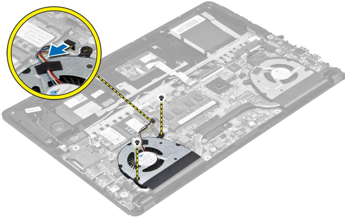
4. Lift and remove the left system fan from the computer.
