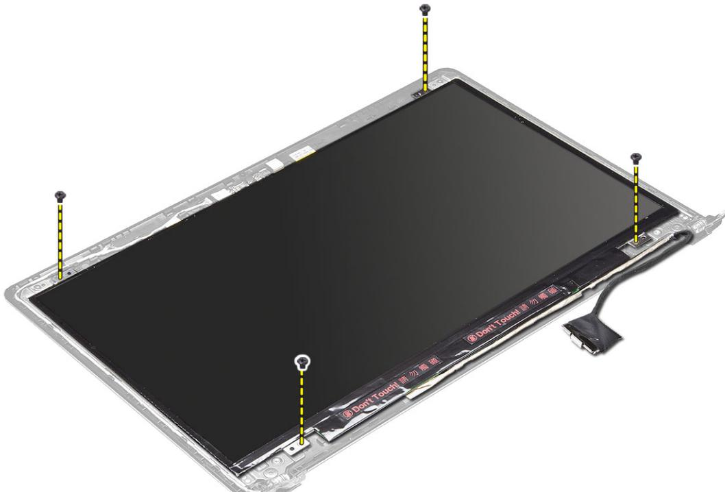
4. Lift and remove the display panel from the display assembly.
