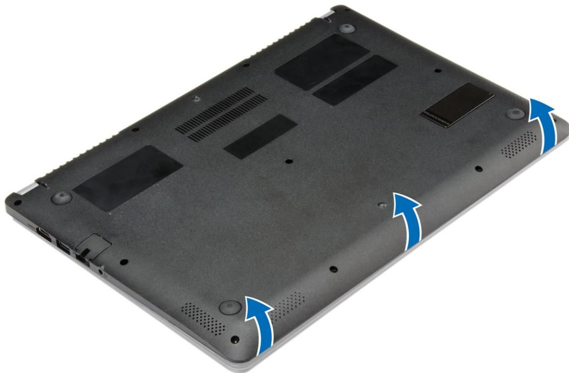
4. Lift and remove the base cover from the computer.
