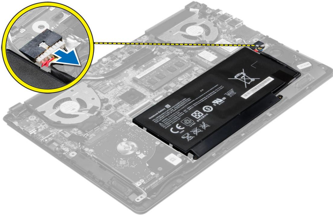
4. Release the tabs that secure the battery in the battery bay.
