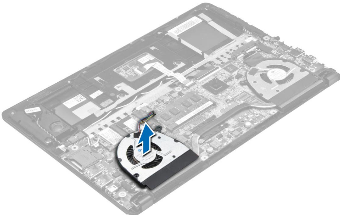
5. Disconnect the right system fan cable from its connector on the system board. Peel away the system board flex cable from the right system fan.
