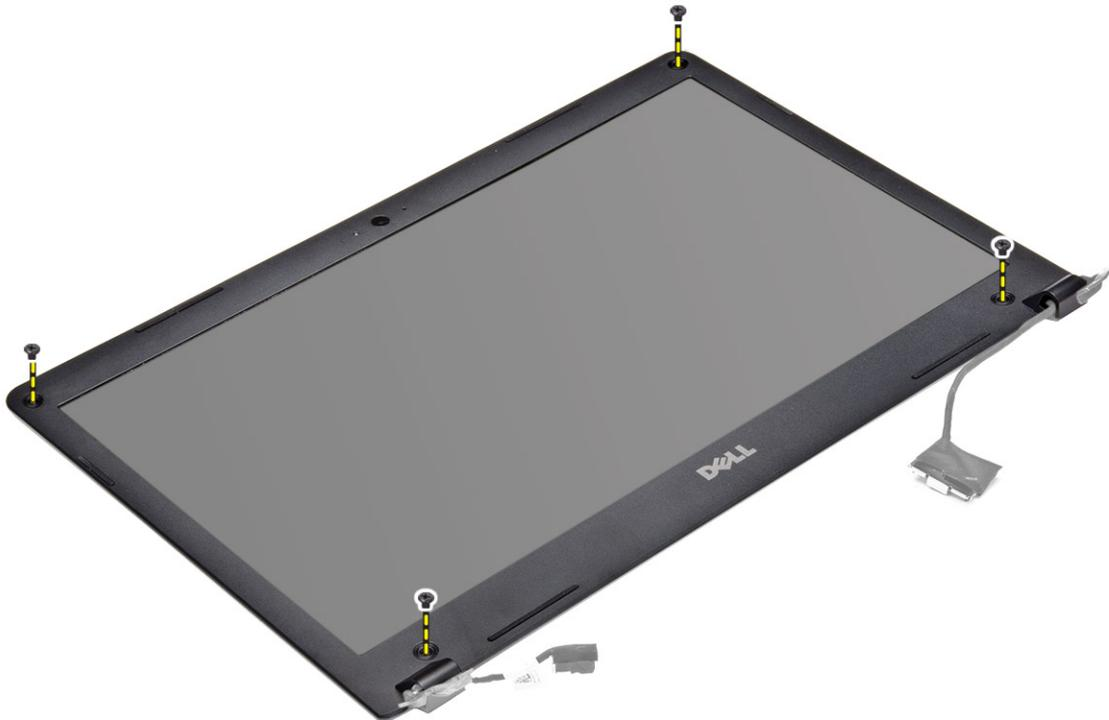
6. Pry along the inner edges of the display bezel and remove it.
