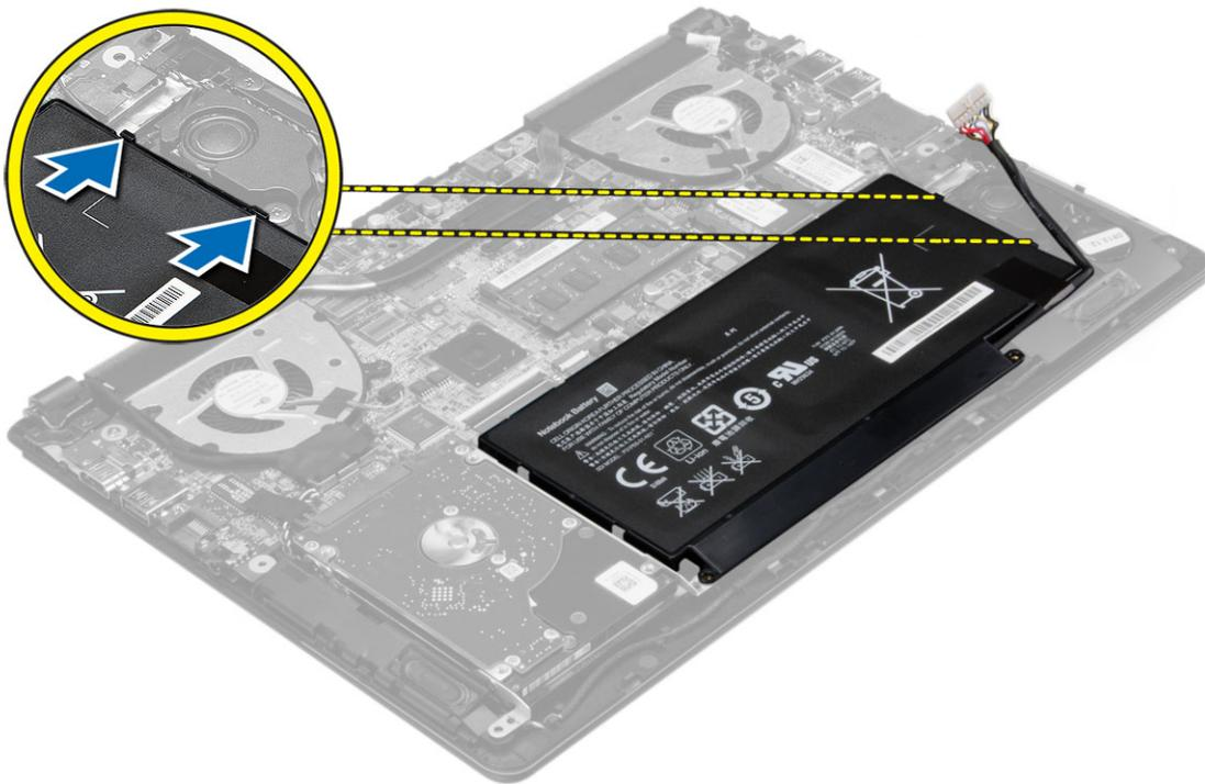
5. Lift and remove the battery from the computer.
