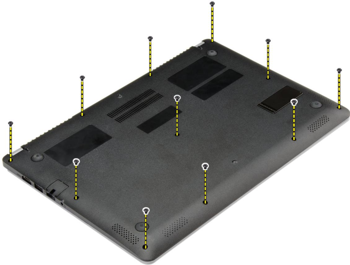
3. Pry the base cover along the edges to loosen it.
